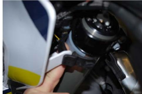
If additional space is required, you can use the gray fork spacers to move the top of your headlight mask out to provide extra clearance.
