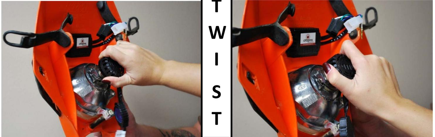
**STEP THREE:** Secure your base to the reflector, with the BA20D it will twist to lock into place. Others will have factory bail wires to hold the base into the reflector. In some cases, you may need to install the base into the reflector and then install the bulb into the base by lining up the tabs and twist to lock the bulb to the base.
