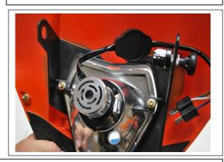
Step Four: Use the appropriate torx driver to remove the top two screws holding the top of your reflector to the mask. Loosen the middle bottom screw but do not remove. Install the supplied bushing to increase clearance between the back of the bulb and your headstock. As shown below: Reinstall your headlight mask to your motorcycle.
