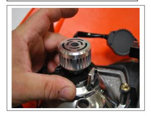
Step Two: Your BA20 D base is fixed to your headlight replacement bulb. After removal of the old bulb to install the new bulb line up the bulb so the power wires are in the facing up or approximately in the 10 o'clock position. As shown below.
