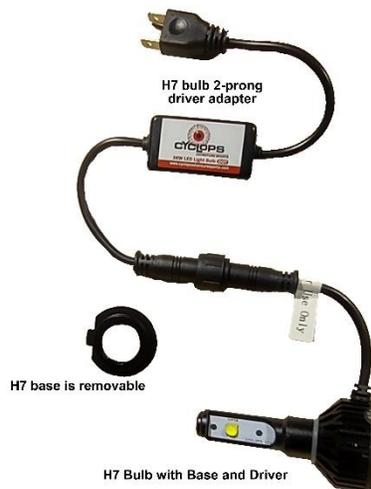
6. Feed the wires and driver into the headlight housing
