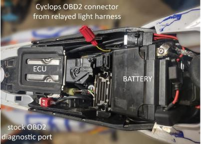
**4.** Run the light-power output wire under the fuel tank and out to a suitable location for the lighting you are installing.
