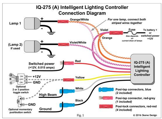
Connect the solid violet and orange wires through an appropriate fuse with a Posi-lock® connector, then to a switched or unswitched 12 volt source. Note that the IQ-275 serves as a relay, so no separate relay is required.
