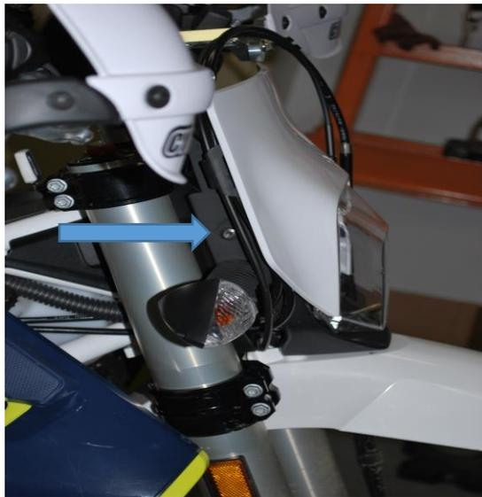
1. Remove the headlight mounting screws (blue arrow above) on both sides of the headlight mask, the headlight can now be removed from the motorcycle.
