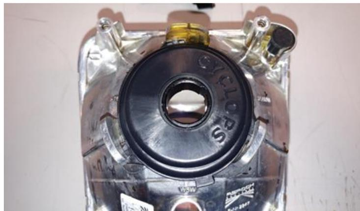
9. Install bulb into metal H4 base with foam dust seal. Make sure to align the narrow and wide keyways. Give slight inward pressure and clockwise twist.
