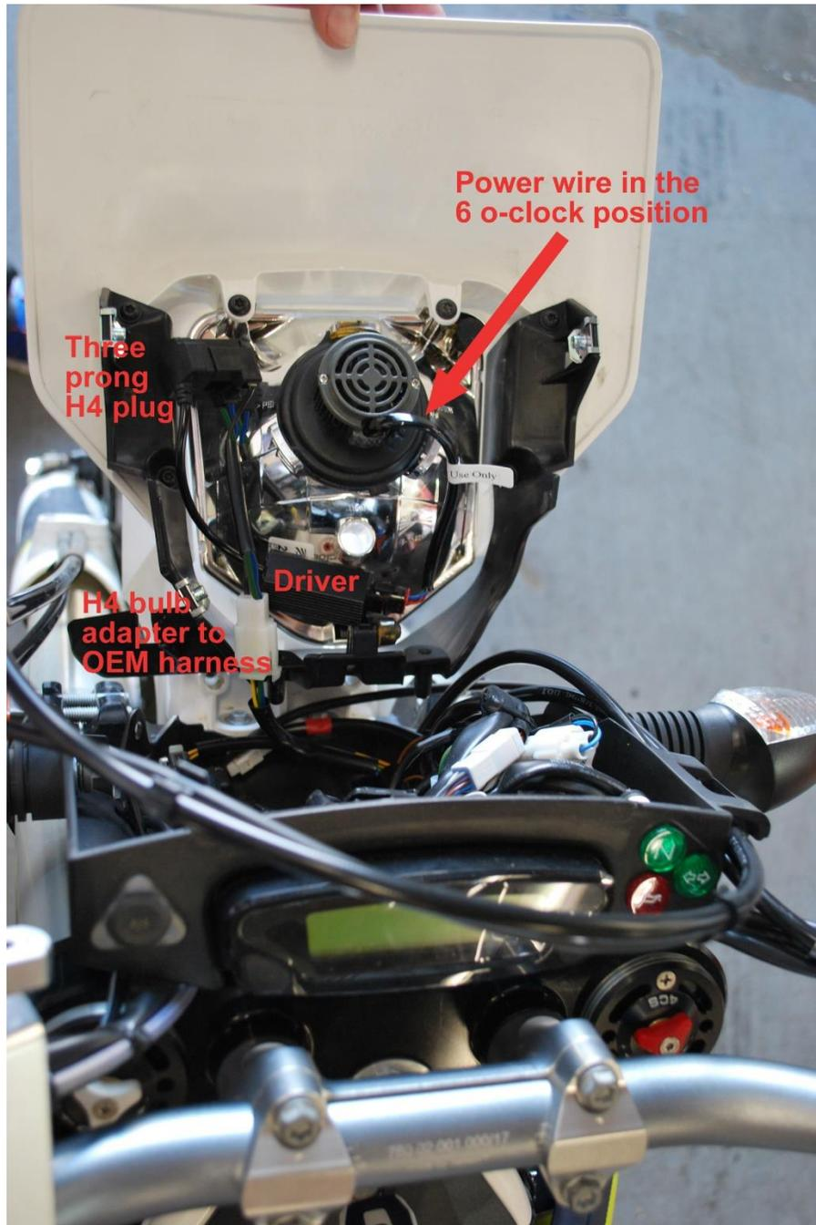
12. Ensure emitters are facing left and right with upper portion of the LED exposed and aim your headlight.
