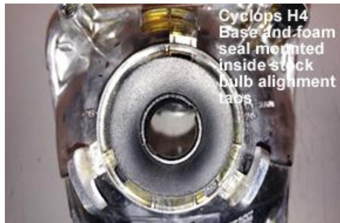
7. Confirm the supplied O-ring is in the Cyclops backing plate.
