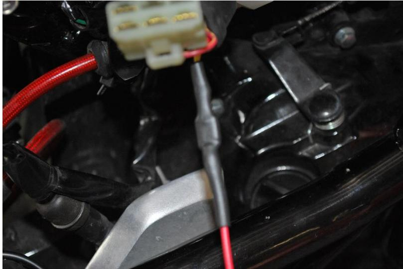
Next run the jumper wire up the side of the frame rail to the plug under the seat that goes to the tail light. This will be a 3 wire connector.
