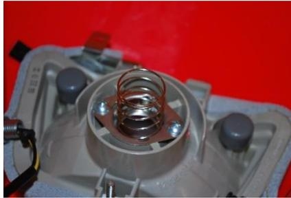
6. Insert bulb into housing. Be sure all three tabs line up before giving a light inward push and a clockwise twist about a ¼ turn, until seated.
