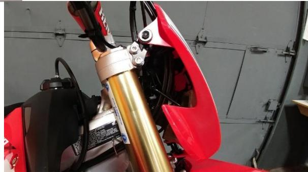
10. Plug bike harness into headlight harness and mount headlight mask.
