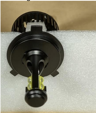
H4 bulb is properly oriented inside the light housing with the emitters facing left and right. The H4 bulb also has a shield below the emitters when properly oriented. The power wire should be in the back at the 6-o'clock position
