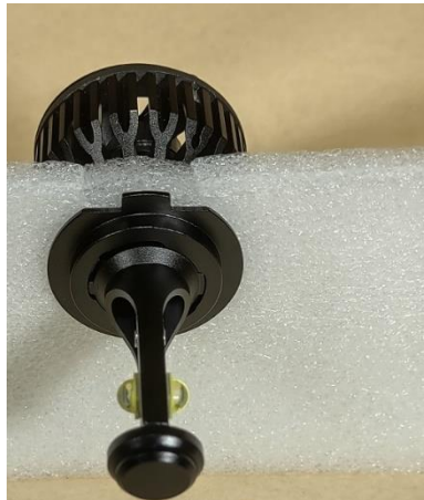
H7 bulb is properly oriented inside the light housing with the emitters facing left and right. The power wire should be in the back at the 6 o'clock position
