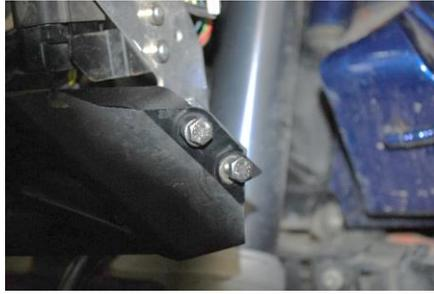
Once satisfied with the fit tighten up the 4 side bolts being careful not to smash the plastic grill attachment points.
